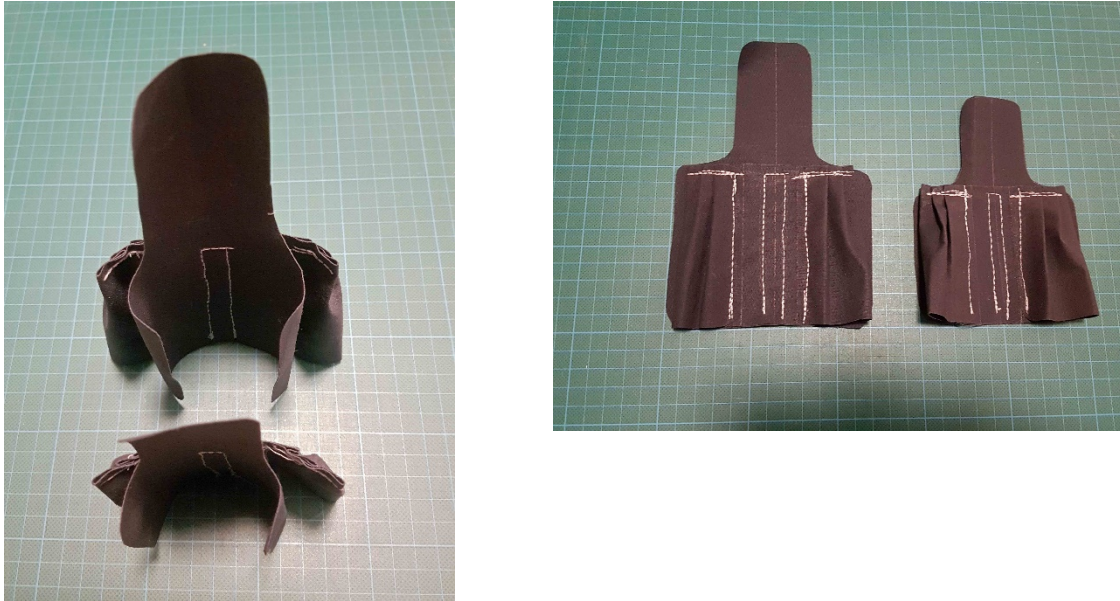
Figure 10: Male and female-sized GPS packs of the new design under construction. They have a larger and smoother contact with the goanna's skin and are easier to sew than any of the previous designs.
