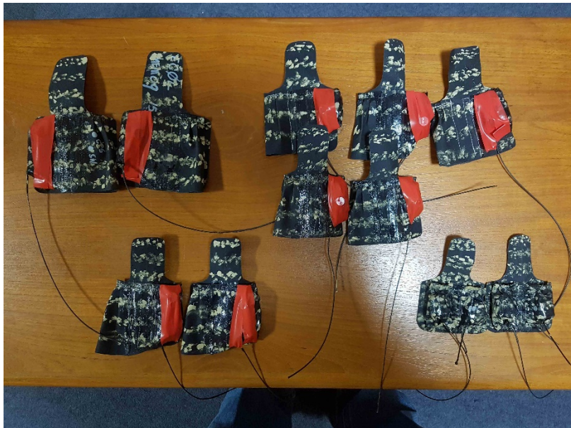
Figure 11: Eleven GPS packs in production for use in the 2021/22 goanna season. This year we have four sizes: male, female, long female and nano. The protruding wire aerials are part the VHF radio beacons used for manual tracking. Red tapes hold magnets in place which keep the radios turned off. These GPS packs will be ready to use after new software has been installed in the GPS devices (not shown), which will then be sewn into the saddlebags on the opposite side to the radios.
