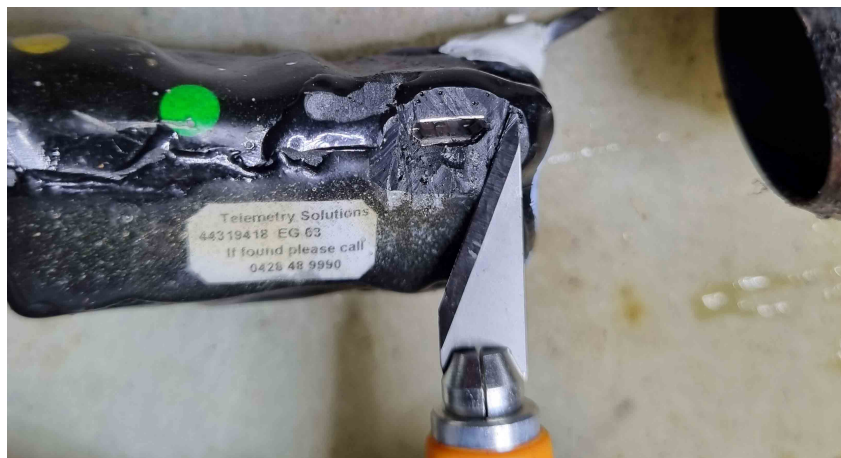
Figure 1: Slicing open a precious GPS unit using a heat gun and sharp blade.
