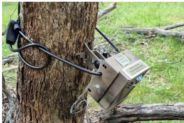
Figure 9: A camera set up at Ainslie-Majura with a steel security box, python lock and labels. This camera is within the view of another camera placed in a nearby tree using a ladder
